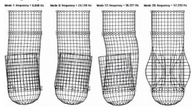
User interface of the version 1.5 of *NewTone* by example: Calculation of coupled (structure-coolant) vibrations of a WWER-type reactor. Postprocessing: Eigen modes
